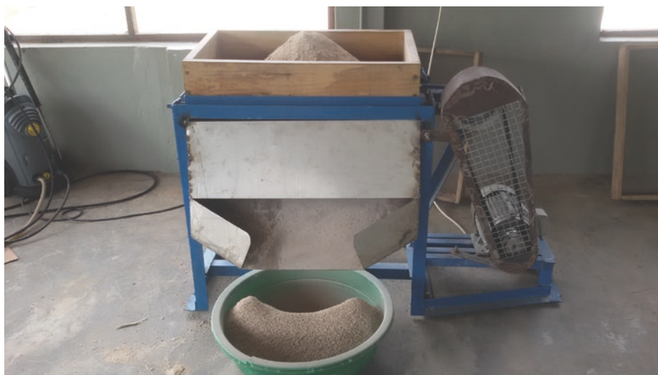
Figure 4 Sieving machine showing fine fraction (in bowl) and coarse fraction (trapped in the hopper)
