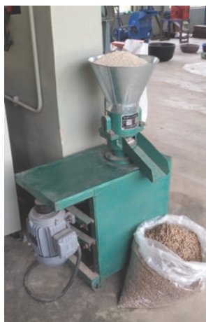
Figure 6 Pelleting machine with loose mash (in hopper) and pellets in the plastic receptacle
