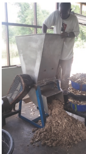
Figure 2 Modified grater for cassava peels
