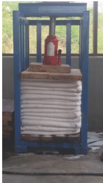
Figure 3 Physical dewatering using a hydraulic press
